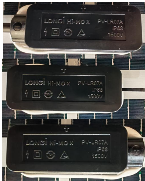
Fig. 5: detail view of closed junction box
